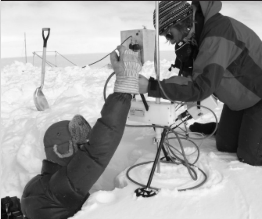
Student researchers use a penetrometer to measure density profiles in a 2-meter pit at Summit, Greenland.
